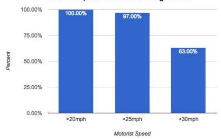
recommended speed, causing danger to cyclists travelling along the blind spot of the road curve. This speed graph shows how significantly more motorists are traveling eastbound at higher speeds compared to motorist speed from the opposite direction. As motorists are driving towards Western Ave, 63% of people behind the wheel are traveling at speeds greater than 30mph, making cycling along this road a serious hazard.
